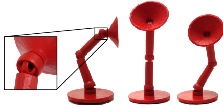
Figure 20: Lamp model printed using joint model from [CCA*12].
